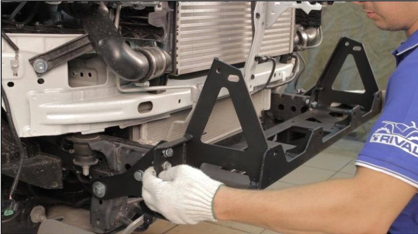
16. Mount winch bracket. Use OE bolts and supplied bolts, nuts, washers from the RIVAL fitting kit bag.
