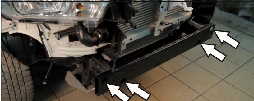
10. Remove 4xM10 bolts fixing crash beam to chassis. Set aside for re-use later on. Remove crash beam.
