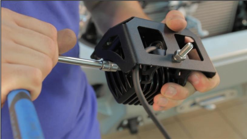
33. LED lights have been mounted to the Bumper Body for transport purposes and are not tightened to the specified tension.
