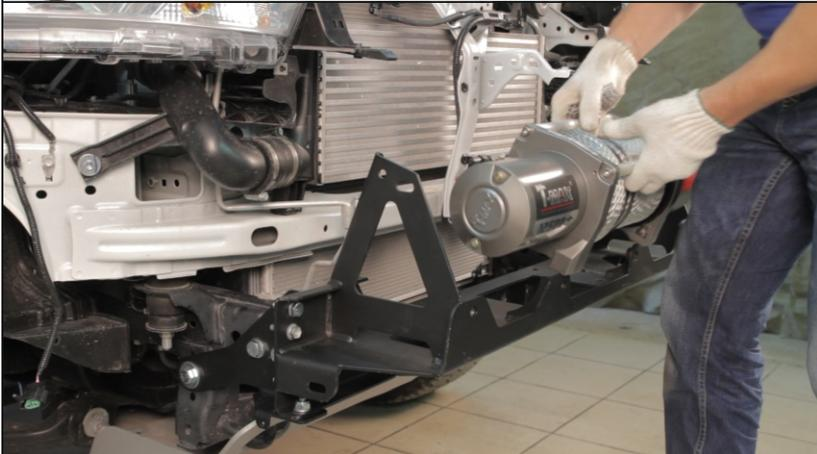
18. Mount the winch. Fix it to the mount with bolts supplied with the winch.
