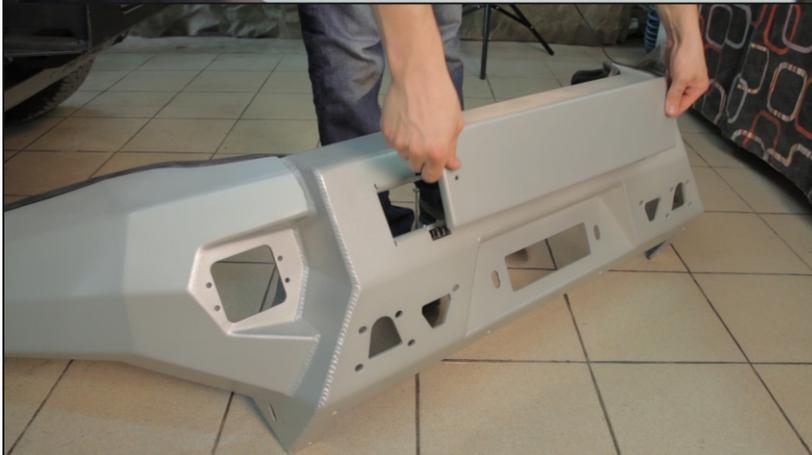
22. Place license plate on the bumper. Fix loops using bolts M6x16. Align loops the in best way.
