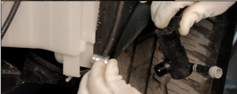
14. Disconnect washer fluid bottle, remove the pump and insert the supplied plug instead (18).
