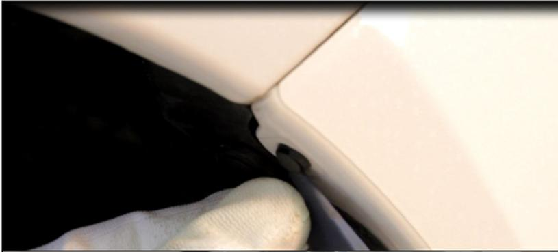
5. Remove all scrivets retaining bumper along inside edge of wheel arches.
