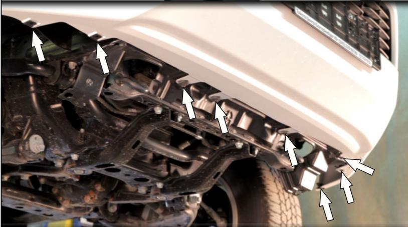
4. Remove lower bumper retaining screws.
