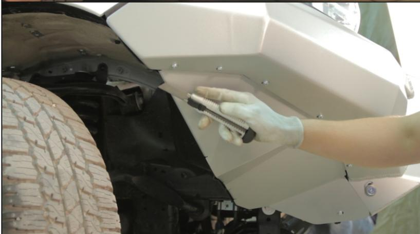
37. Push flap to plastic fender and mark cutting line.
