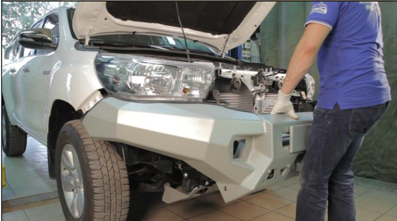
24. Install bumper body onto the winch bracket.
