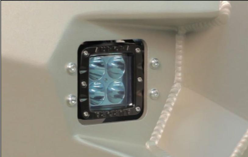
34. Install brackets with LED lights. Fix them with M6x16 round-head screws (26) and M6x12 washers.
