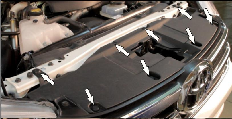
1. Open the bonnet and remove all scrivets holding the grille in place.
