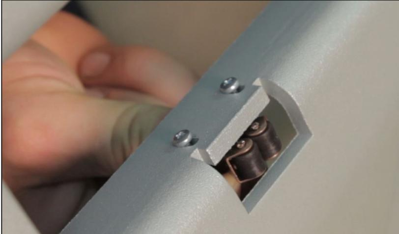
20. Mount roll latch (40) to bumper with screws M3x12 (25) and nuts M3 (30).
