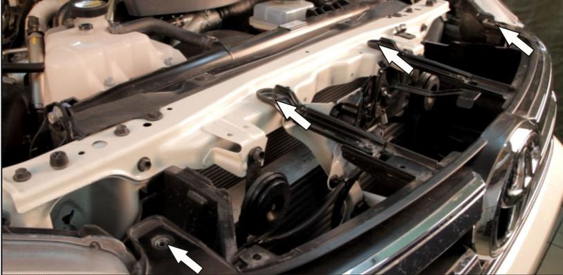
2. Remove upper grille retaining screws.
