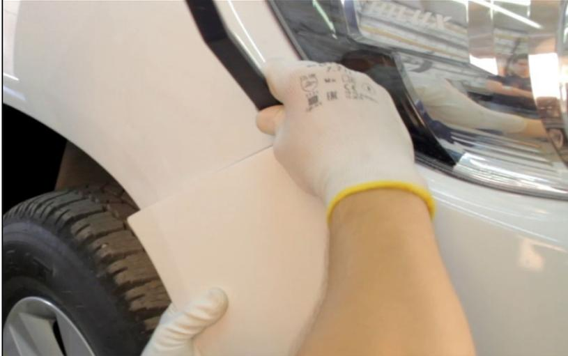
6. Carefully remove bumper from vehicle by pulling on each side of the bumper near the wheel arches and working your way towards the centre.
