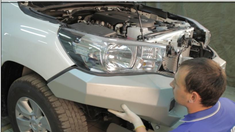
28. Adjust bumper to reach an equal gap to the vehicle body on both sides. The gap should not be less than 18mm. A gap between the headlights and the rubber profile is acceptable.
