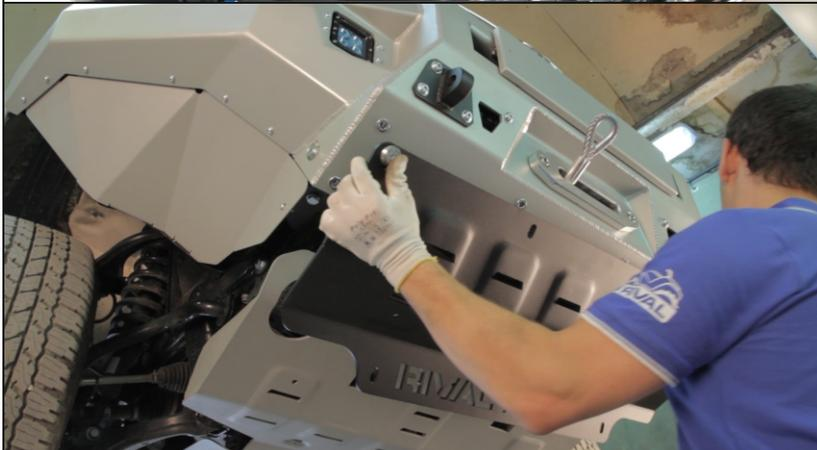
42. Install middle plate (10) between bumper and RIVAL skid plate. Fix it using 9x M10x30 countersunk-head screws (28) and countersunk washers (19).
