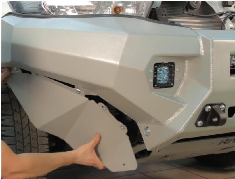
36. Install flaps using few M6x20 round-head screws and M6x12 washers.
