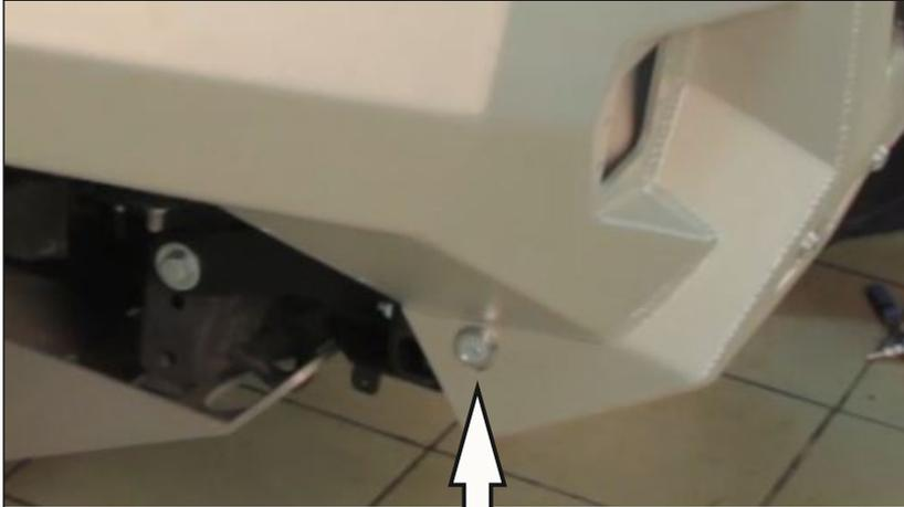
27. Place bumper body to the winch bracket using M10x30 countersunk-head screws (28), countersunk washers (19), M10x30 washers (37) and M10 nuts (32). DO NOT TIGHTEN YET.
